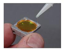
Position the new lens in the mount. Make sure it is facing the right direction. The lens should be sitting flush in the lens mount and not at an angle. Use three small spots of the Optic Mounting Adhesive. Do not over apply the adhesive. The adhesive is specially formulated for mounting laser optics and should not be substituted. The mounted optic will be ready for cleaning and use in 1 hour.
