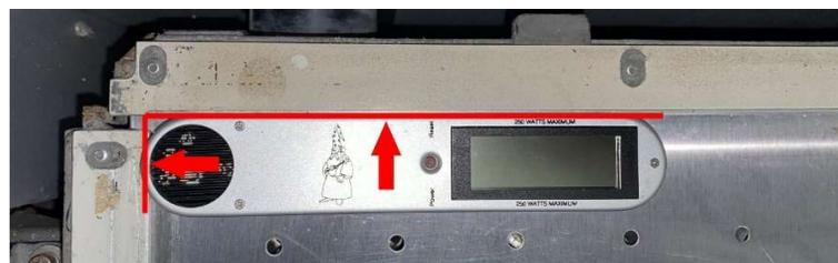
2. Adjust the focus of the laser to the surface of the laser target.
