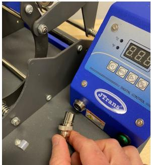
• Loosen the thumb screws of the heat wrap from the mug press chassis, then remove the heat wrap from the press chassis.
