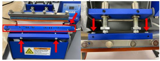
• Place the mug press attachment onto the long blue bars. Attach the wrap to the blue bars using the provided thumb screws.
