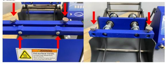
• Use a Philips head screw driver to screw in the replacement long screws provided with the mug press attachment into the mounting holes on the front of the chassis. Place the remaining replacement long screws into the horizontal mounting holes on the back of the press chassis. Only tighten/place the screws enough to be held in place temporarily.
