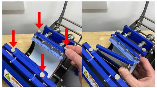
• Use a Philips head screw driver to completely remove the two mounting screws located on the front of the wrap mount. Also completely remove the thumb screws from the front and back of the press chassis.
