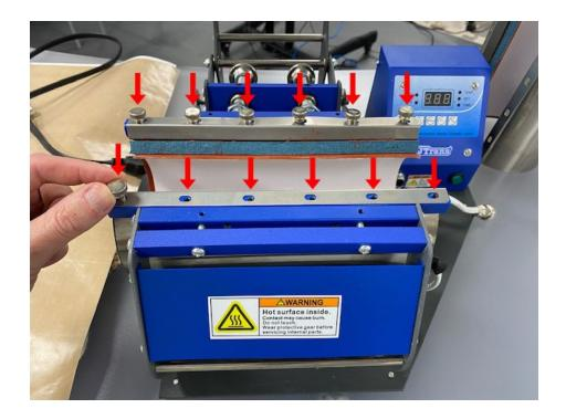
• Plug the mug press attachment cord into the socket of the mug press display and screw in the set screw until it is snug.
