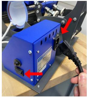
• Remove the current mug press attachment by loosening the set screw and disconnect the heat wrap cable from the mug press display box.
