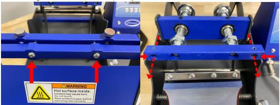
• Place the two long blue bars provided with the mug press attachment on the front and back ends of the chassis. Use a Philips head screwdriver to finish screwing in the long screws on the front and back of the press chassis into the bars until they are snug.
