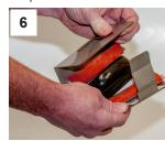
**Remove -** Slide the prong clasp out of the loop clasp to remove the substrate.
