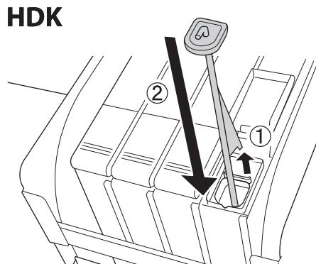
**Caution:** Press the ink inlet cap down firmly. If the slider comes into contact with the ink inlet cap when pulling it out, the cap could get damaged.
