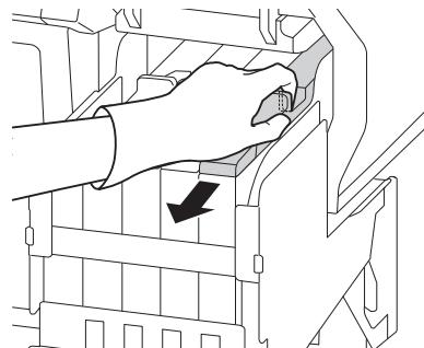
**Caution:** Do not tilt the slider. If the chip unit is dropped, it may break.
