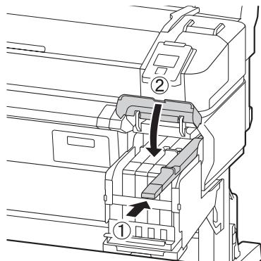
**Caution:** Do not push the slider in with too much force. Failure to observe this precaution could damage the printer.
