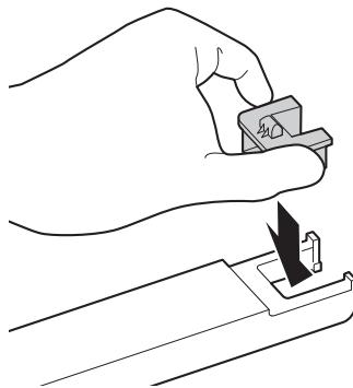
6. Hold the slider level horizontally and insert it. Close the ink tank cover.
