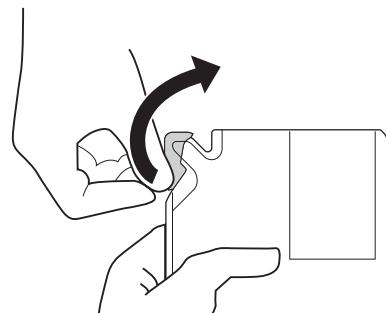
11. Insert the spout of the ink pack into the groove and slowly tilt it to pour the ink.
