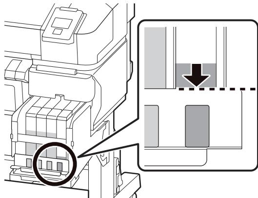
If the remaining ink level is above the top edge of the metal plate or greater than 1.9 in. (50 mm) from the base of the ink tank, continue to use the printer until the remaining ink level is 1.9 in. (50 mm) from the base of the ink tank so that you can use all the ink in a new ink pack to refill the ink tank.
