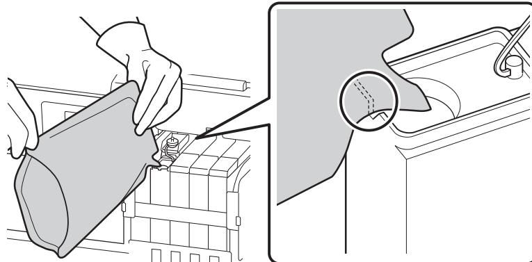
**Note:** Be sure to completely empty the ink pack into the tank. Do not use an ink pack to refill multiple ink tanks. This can prevent the proper display of messages from the remaining ink warning system.
