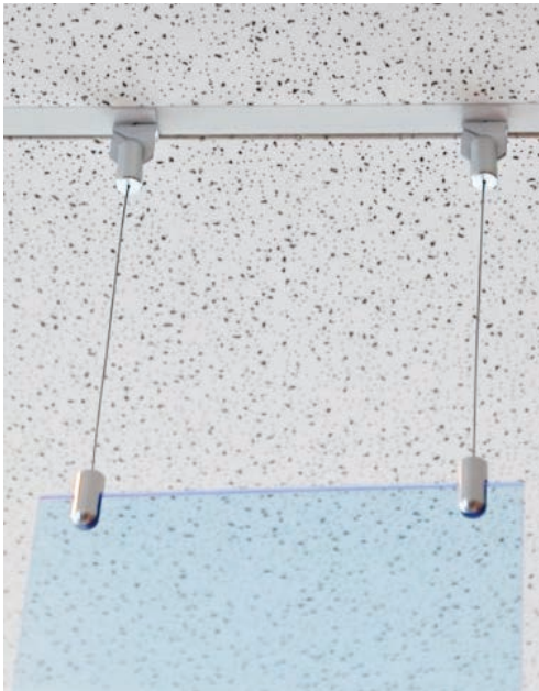
Drop Ceiling Wire Suspension Kit Two acoustic panel t-track clips Two vertical grippers One 10' span of 3/64" wire Four panel grippers.
